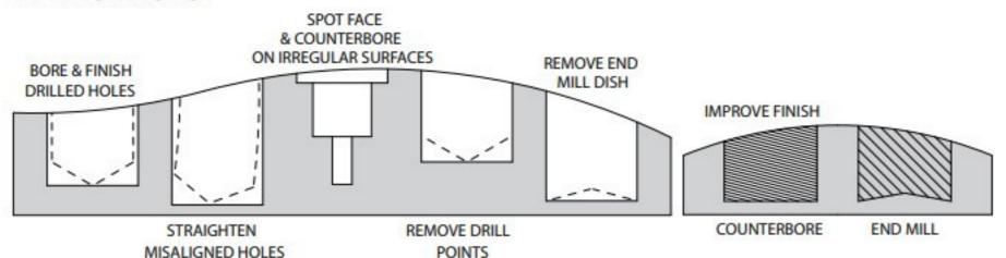
removes end mill dish or drill points while effectively spotting on irregular surfaces.
