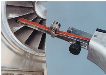
Efficiently rework turbine blades with specialized contact arm.
