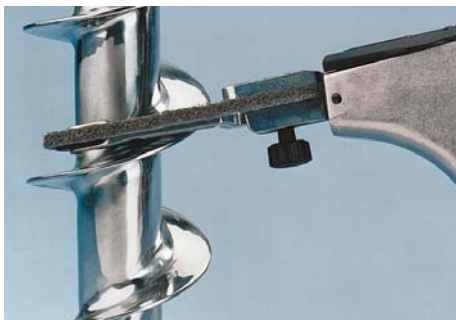
Clean and finish using non-woven nylon belts.
